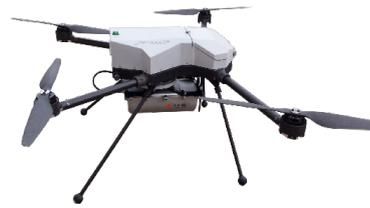
SPIR-Explorer Sensor mounted on an AERACCESS drone
