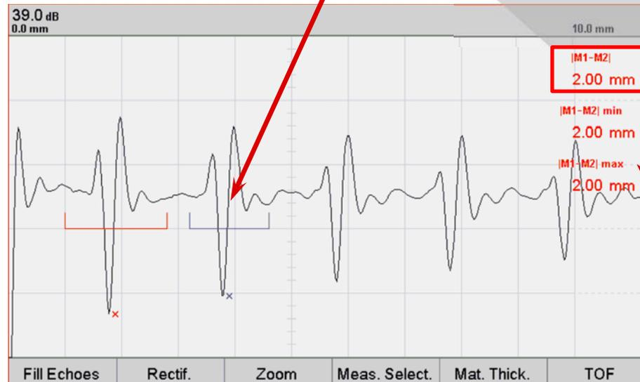
Min / Max – storage of wall thickness data
